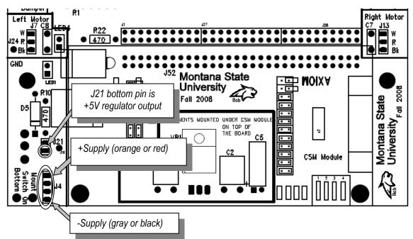
Connect the positive (red) wire from the supply to the red (or orange) wire of the pigtail using a banana cable and alligator clip. Connect the neutral (black) power supply wire to the black (or gray) pigtail using another banana cable and alligator clip.
