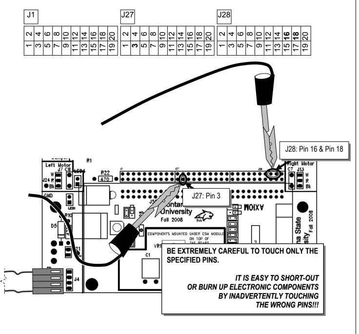
$\rightarrow$  Finally, keep the grounded wire on <u>J27 pin 3</u> and move the other grounded wire to <u>J1 pin 19</u>. Note that **J1** pin 19 controls the decimal point.
