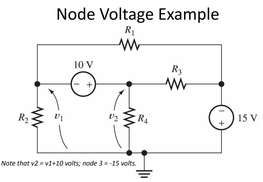
Problem: voltage source s do not constrain current, so how do we write KCL? Need to use "supernode" concept.
