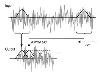
Figure 2: Simple time-domain block downsampling procedure.
