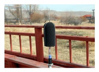
Figure 4: Windscreen (32cm x 10cm) and bird spike enclosing microphone
