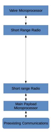
Design Alternative 2: Microprocessor with amateur radio link.
