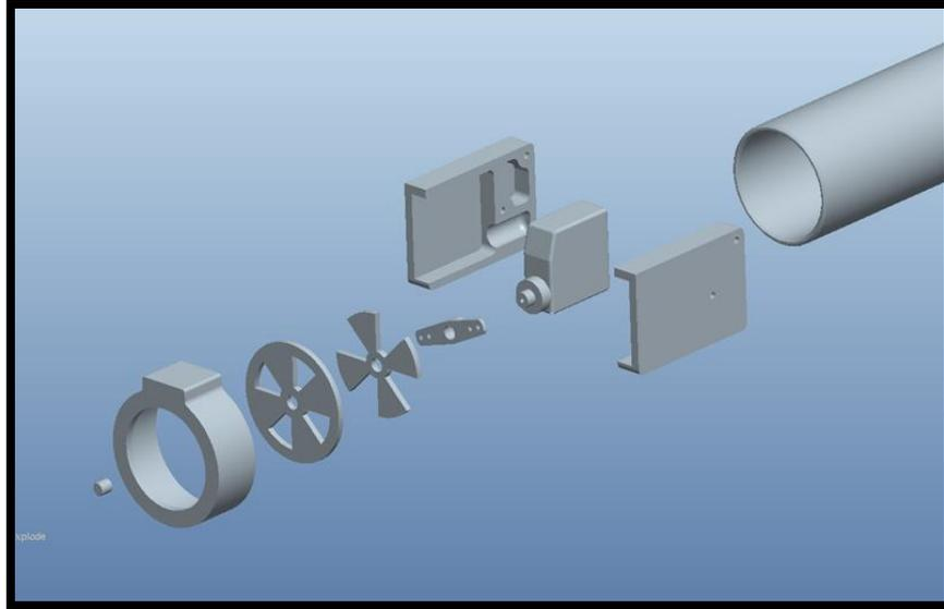
Figure 1: Exploded CAD model of the Valve geometry
