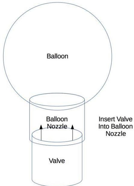
**Mechanical interface: inserting valve hardware into latex weather balloon** - The mechanical interface between the customer's latex weather balloon and the valve assembly requires the user to mechanically insert the valve sub-assembly into the balloon nozzle. Once the valve has been inserted to a reference mark the customer must secure the valve to the balloon using zip-ties or other similar means.
