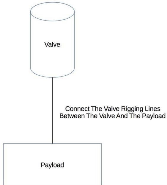
**Mechanical interface: connecting rigging lines to the valve and main payload** - The mechanical interface between the valve and main payload requires the user to physically couple their payload to the helium valve hardware. The rigging lines used will be provided by the customer however our product will provide hard mounting points to securely attach these lines to the valve.
