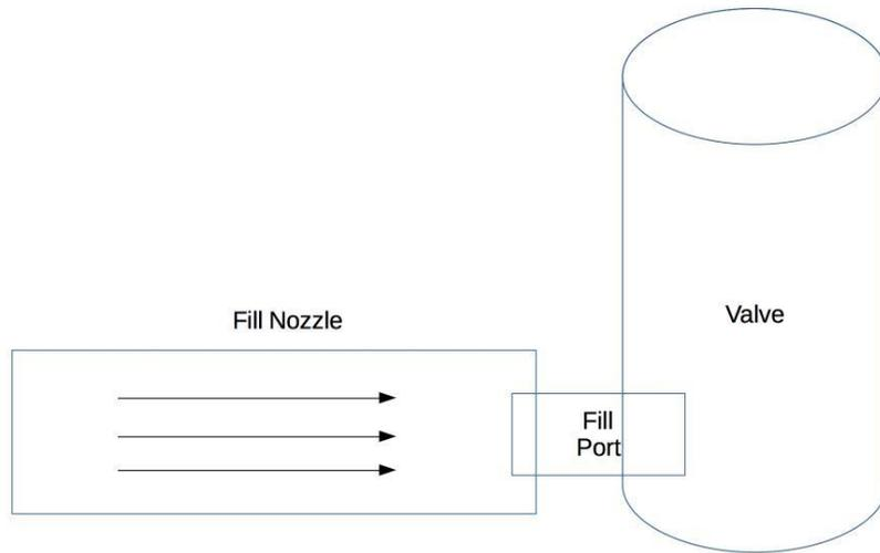
**Mechanical interface: attaching helium fill nozzle to the valve fill port** - The mechanical interface between the fill nozzle and fill port requires the user to physically connect a fill nozzle from their helium tank and regulator to the fill port of the valve assembly. The user must then operate their helium filling equipment to fill the latex weather balloon as needed.
