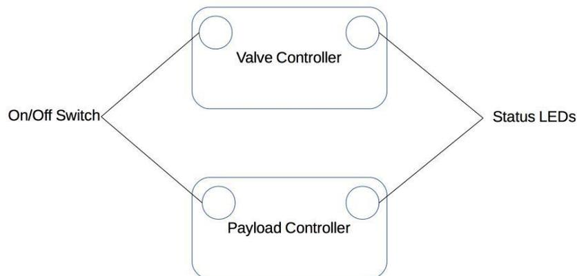
**Mechanical interface: turning on the valve electronics and verifying status** - The valve electronics require a mechanical interface between the user and the product activation switches. The user must physically actuate the power switch to turn on the valve electronics. Once the electronics have powered up the user must verify proper operation using status LEDs located on the valve hardware.
